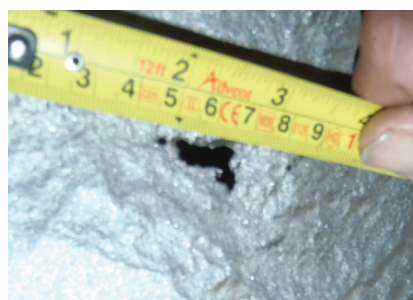
Defect > 12.5\text{mm} ( \frac{1}{2} " ), not covered by standard design
